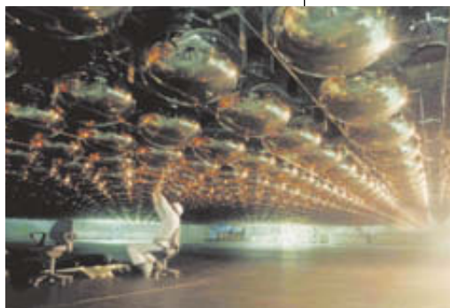
PHOTOMULTIPLIER TUBES installed in the roof of Super-Kamiokande during construction in 1995.
